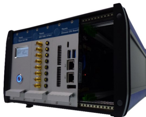
Fig. 3: TSEP Themis with IEEE 1588 Trigger multiplexer
