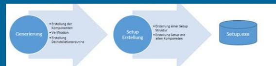
The Installation Creation Tool helps the user to compile all the installation files and finally convert them into an executable set-up. In this case, a database is created from the input data (ie configuration files, installation files) from which a setup is created after verifying all installation steps.
