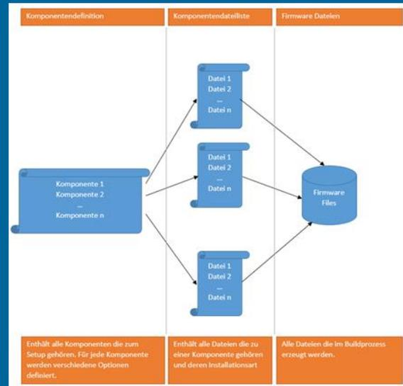
For large installation packages, TSEP Kratos is used at customers with set-ups up to 1 GB, the Installation Creation Tool supports the user with a large number of checks and monitoring. This way, duplicate files are detected and eliminated, or incorrect path information and missing files are communicated to the user.
