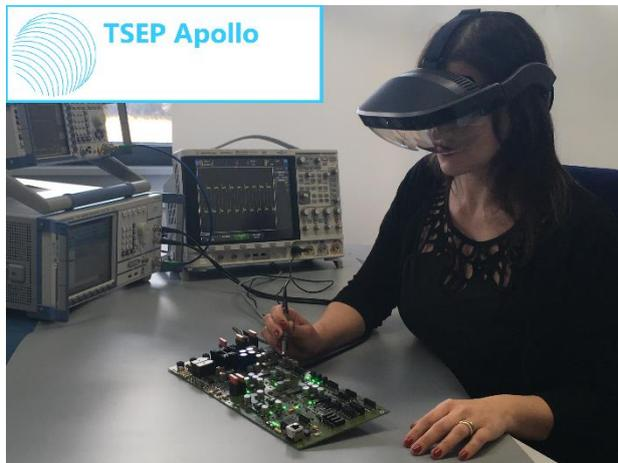
TSEP Apollo does not rely on a proprietary approach to the control of AR glasses, but uses the established standard OpenVR. Thus, all common AR glasses can be controlled. The customer can optimise TSEP Apollo for his preferred model.
